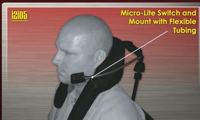
Includes: i2i780, Swing-Away ([SUS9-L] Left) with a Flex Micro-Lite Mount (**CN600**) and a Micro-Lite Switch (**ML210**).
