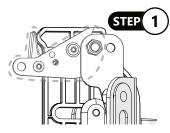
This represents the locked position of the hardware. Before operating the wheelchair, make sure both latch assemblies are locked in this position.
