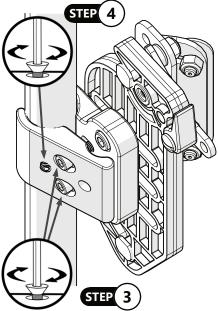
4. Adjust the mounting hardware for height on the cane, and tighten the two M5 x 0.8 x 22mm Socket Head Screws (A) to secure it in place.
