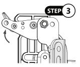
Lift the latch to release the pin and allow the back support to be removed.
