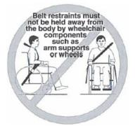
Belt restraints should not be routed outside of the wheelchair, over the wheelchair wheels, or over the wheelchair arm supports and should not be held away from the body by wheelchair components or parts.
