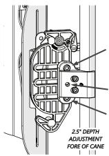
There are three M6 x 1.0 x 25mm Socket Head Screws (E) holding the cane clamp to the QR Pro Main Plate (I). One of these screws is located underneath the outer clamp, but a hole has been provided to loosen it enough to perform a depth adjustment. Fit the 4mm hex wrench through the hole and into the top of the socket head screw to loosen or tighten it, respectively.
