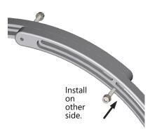
The support arm has two ranges: short to medium, and medium to long. The screws must be removed to place the halves in the other range. If the support arm is not in the proper range for your installation, just remove the screws holding the halves of the support arm together, and reinstall them in the other slot on both halves.
