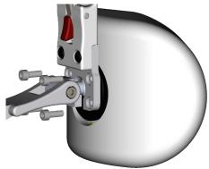
**Step 4** - Ensure the split ring is parallel with the ring mount and the socket head screws are sufficiently tight to secure the headrest pad and Anterior Head Support in position.
