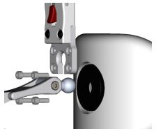
**Step 2** - Place the split ring adapter of the Anterior Head Support behind the 17mm ball and align the four holes with the four threaded holes in the mounting ring of the headrest pad.
