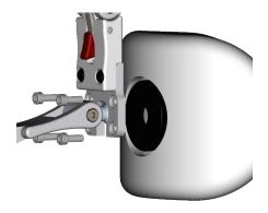
**Step 3** - Install the four socket head screws to secure the split ring to the ring mount on the headrest pad. The socket head screws should be tightened in a pattern to maintain alignment of the split ring with the ring mount. They should be snug, but do not overtighten them, as this can cause damage to the 17mm ball or mounting surfaces.
