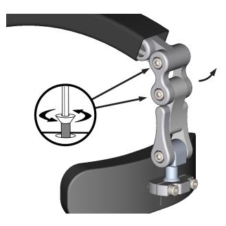
To adjust the forehead pad for depth, loosen the socket head screws at the junction(s) you wish to adjust.
