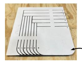
2. Place the Base Foam (D) on a flat assembly surface, paper side up, and align the Sizing Template radius as shown in the image to the left.
