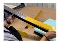
Locate the two Adductor Wedges (H, J). There will be two adhesive-backed sides on each wedge. Peel the protective paper off of the side adjacent to the right angle on one of the adductors.
