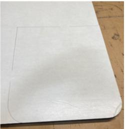
5. Peel the paper adhesive protector from the base foam exposing the adhesive surface. Return the base foam to the assembly surface, adhesive side up.
