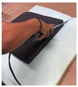
10. Flip the assembly onto the open cell foam layer and trim the excess foam along the straight edges of the base foam layer. Following the edge of the radius on the base foam layer, trim the excess open cell foam from the assembly.
