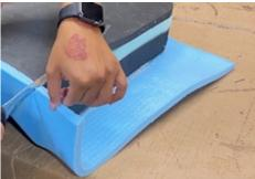
21. Once the bottom, front edge has been trimmed, continue trimming the excess foam from around the edges of the cushion. Follow the curves and contours of the cushion to achieve a straight, smooth appearance.
