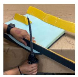
13. Using the electric knife, or other foam cutting tool, trim the adductor wedges to follow the rounded edge of the rear of the cushion.
