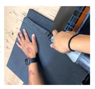
Trim the excess foam to match the side and front edge of the base foam (see above).
