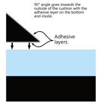
14. Peel the adhesive layer from all surfaces to begin the middle layer assembly.
