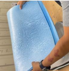
19. Align the edge of the foam with the rear edge of the cushion and slowly lay it forward to the front edge of the cushion. Press firmly to affix the adhesive on the top surface of the cushion.
