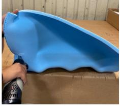
20. Waterfall the Extra-Soft Sunmate (A) over the front edge of the cushion and press it firmly into the other foam layers. Using your electric knife, or other foam-cutting tool, trim the excess foam from the bottom front edge of the cushion.
