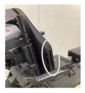
**2.** Slide the angled 125° lateral mounting bracket in behind the square plate in the lateral cover slot
