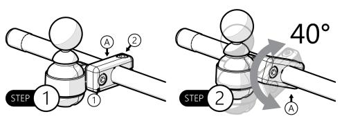
**Step 1:** Loosen both screws (1 and 2).
