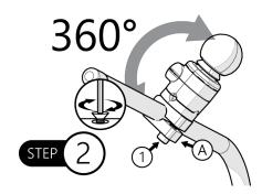
**Step 2:** Rotate block (A) in a 360° range to the desired angle. Tighten screw (1) again.
