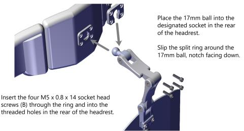
Tighten screws with an M4 hex key, ensuring the screws are tightened evenly and that the split ring is parallel with the mounting plate on the other side of the 17mm ball.
