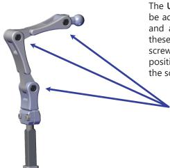
The UniLink Head Support Hardware can be adjusted in three planes: depth, height and angle. To adjust position in any of these planes, loosen the appropriate M5 screw using an M4 Hex Key. Change the positioning of the link(s) and hand-tighten the screw(s) to secure the setting.
