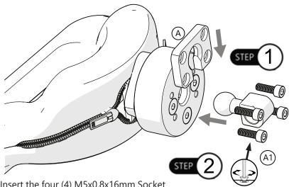
**Step 2:** Insert the four (4) M5x0.8x16mm Socket Head Screws\* (A1) through the split ring and into the Tone Deflector Interface Ring (A). With a hex key, tighten and secure screws evenly, maintaining the split ring's parallel alignment with the interface ring.
