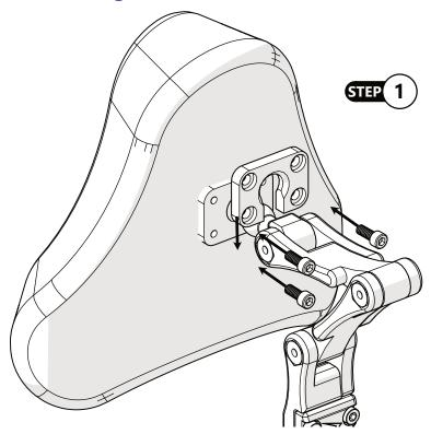
**STEP 1:** Place the 17mm ball in the socket located at the rear of the headrest. Slide the split ring over the shaft behind the ball and then towards the headrest to retain the ball.
