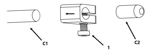
**Step One:** Remove bar plug (C2) from Gatlin arm (C1). Loosen clamping screw (1). Slide clamp onto the arm (C1)
