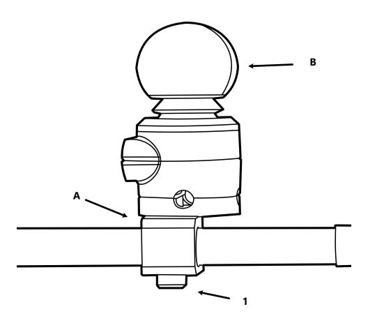
**Step Three:** Tighten the screw (1) with a 4mm hex key, taking care not to overtighten. Mount Multi Joystick (B) and tighten to clamp (A).
